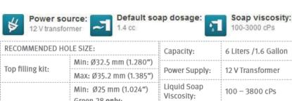
Green 28 only: Min: Ø20 mm (0.78") MF deck mounted soap dispenser: Max: Ø29mm (1.181") Green 28 only: Max: Ø24 mm (0.94") Min: Ø23 Mm (0.906") MF wall mounted soap dispenser:
